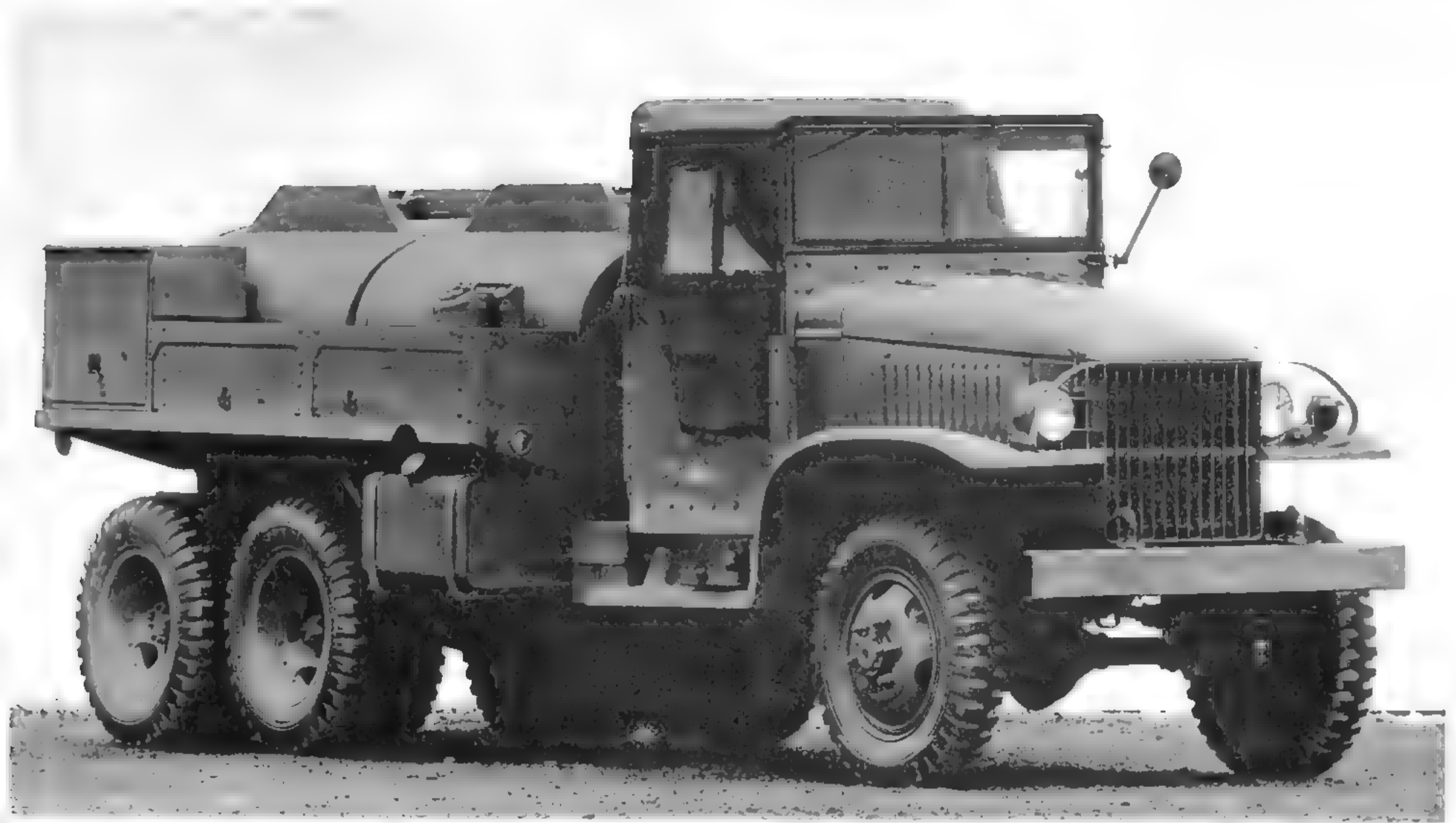
By 1944, GMC was still building fuel tankers, but there had been subtle detail changes, including fitting an open cab. (U.S. Army photo)
